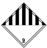
Use Class 9 Miscellaneous Dangerous Goods and UN Identification labels for transportation of lithium ion batteries which are assigned Class 9. Refer to relevant transportation documents. Lithium and lithium ion cells and batteries are regulated in the U.S. in accordance with Part 49 of the Code of Federal Regulations, (49 CFR Sections 105-180) of the U.S. Hazardous Materials Regulations.
